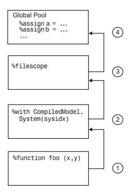
The rule for nested file scopes is similar to that for nested function scopes. In the case of nested file scopes, only the innermost nested file scope is searched.
