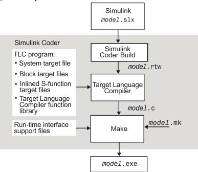
The Target Language Compiler (TLC) is designed for one purpose — to convert the model description file model.rtw (or similar files) into target-specific code or text.
